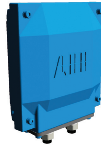
Auxiliary cast iron terminal box Frame size for motor sizes 160 - 250 (variant code 418): 119 x 170 mm, max. 18 strips. No earthing.
